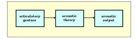
As a preliminary then to articulatory synthesis the actual speech output from the device can indeed be generated from a formant synthesiser which is immediately preceded by the rules of the acoustic theory, thus:
